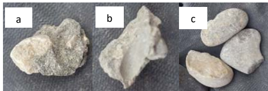
Fig. 1. a) Old mortar attaching to aggregate b) Old mortar as aggregate c) broken Natural aggregate
