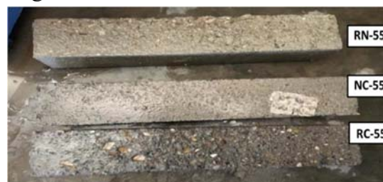
Fig. 4. Damage of specimens after 300 freeze-thaw cycles
