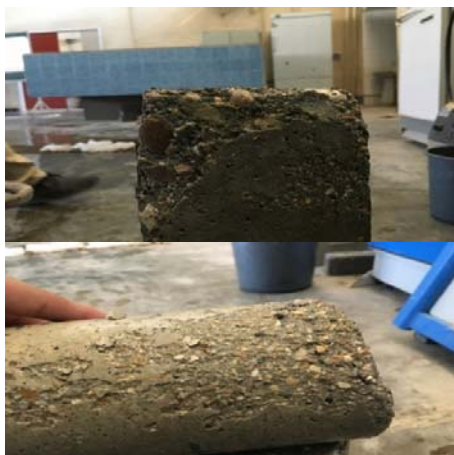
Fig. 5. Damage of corner areas of specimens after 300 freeze-thaw cycles
