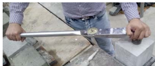
Fig. 2. Twist-off in-situ Test.
