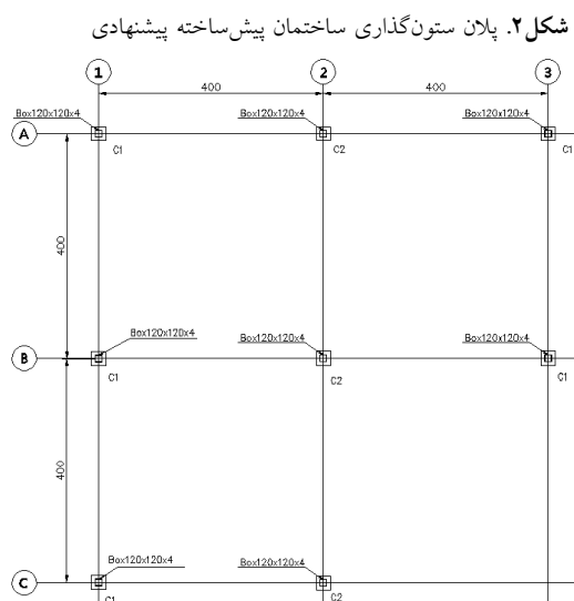
Fig. 2. Column plan of the proposed prefabricated building
