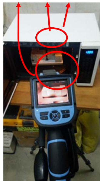
Fig. 2. Microwave, concrete sample and thermal camera
