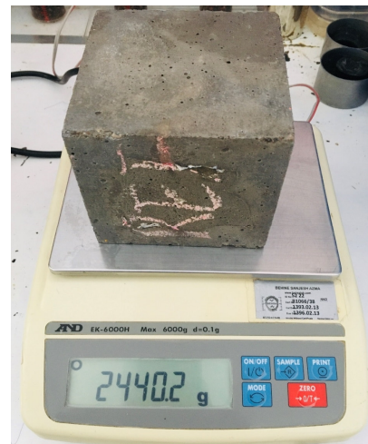
Fig. 4. Weighing the samples to evaluate the amount of water absorption
