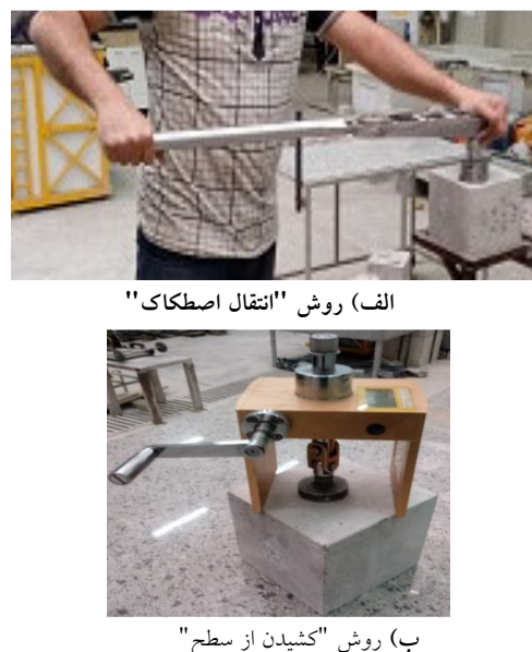
Fig. 3. Evaluation of the compressive strength of mortars
