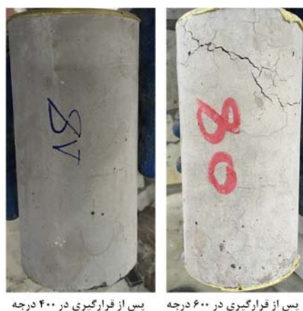
Fig. 5. Appearance of SF-5-1 specimens after heat exposure
