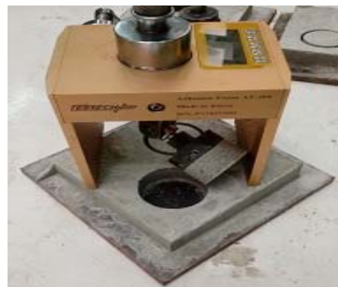
Fig. 4.b. Evaluation of tensile bond strength.
