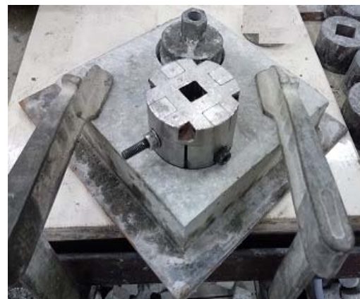
Fig. 4.a. Evaluation of shear bond strength.
