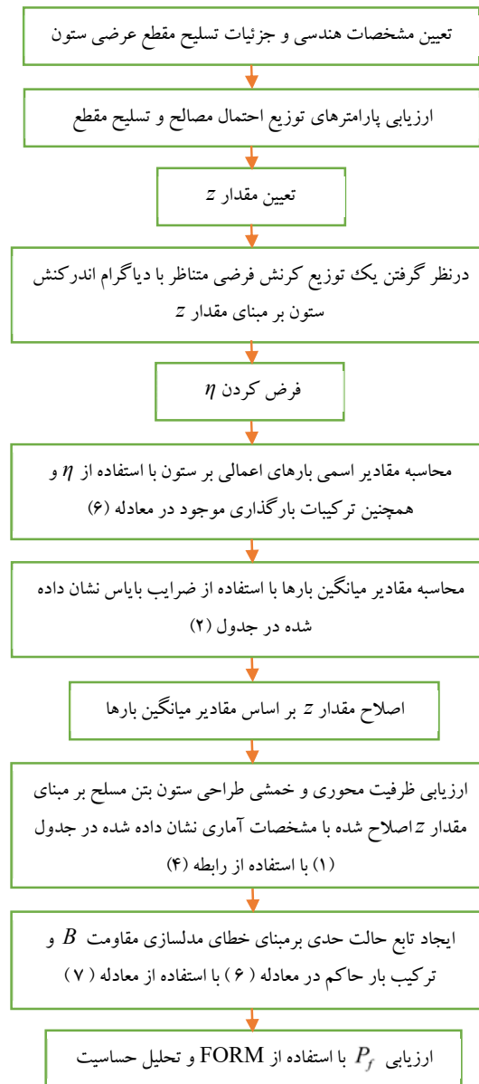
Fig. 5. The Proposed chart of column P_f assessment for the assumed strain distribution.
