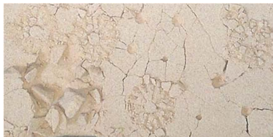
Fig. 5. Photographic of crustal sand layer with MICP
