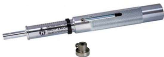
Fig. 3. Pocket Penetrometer and Adapter foot for compressive strength assessment of crustal sand layer
