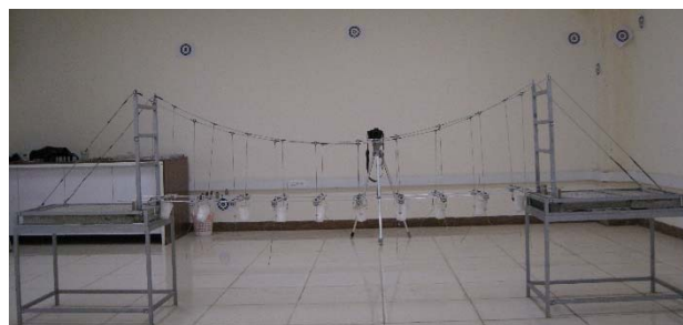
Fig. 3. Real Image of Scaled Laboratory Bridge;
