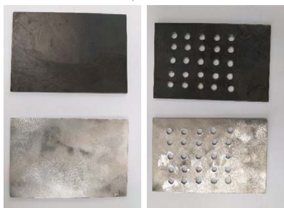
Fig. 2. Perforated and nonperforated iron and aluminum electrodes
