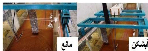
Fig. 3. Groins on the side of the canal and obstacles in the middle of the canal
