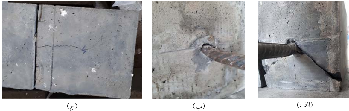
Fig. 6. Failure of the specimens. a. formation of the failure wedge under the bar in the specimen B2, b. local crushing and separation of a piece of concrete under the bar in the specimen B3. c. development of the vertical crack from the top of the bar to the upper face along the bar in the specimen B4 (image of the upper face of the block).
