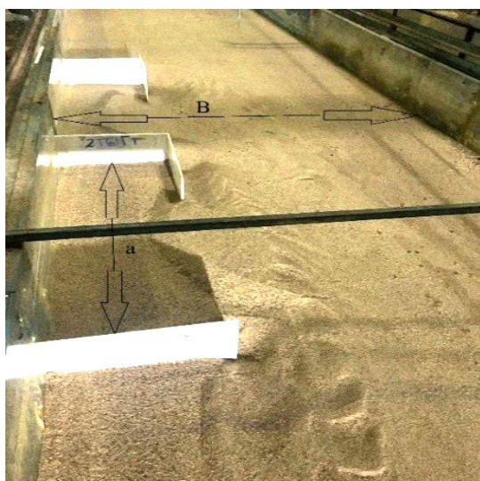
Fig. 3. Spur dikes design for test P4 in flume
