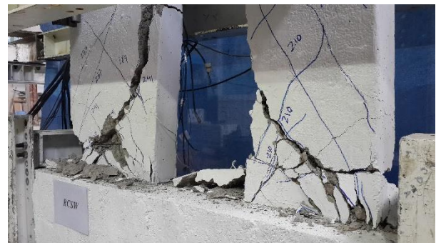
Fig. 11. Concrete failure in wall and wall pier
