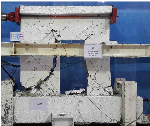
Fig. 10. Cracking pattern on drift 4.0%
