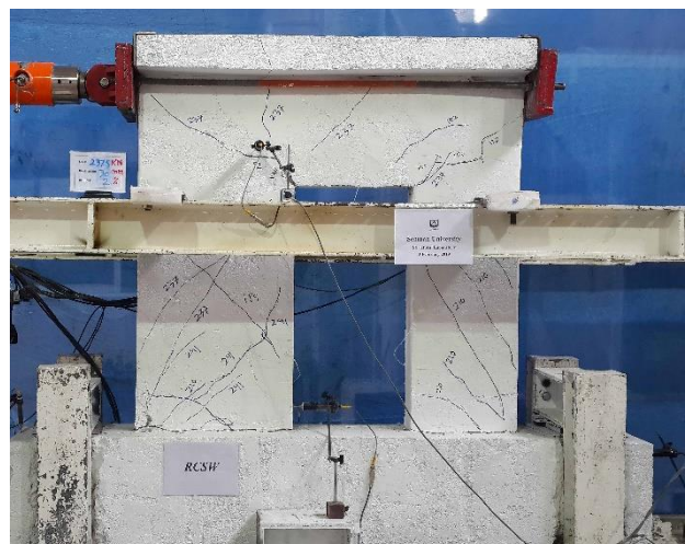
Fig. 9. Cracking pattern on drift 2.0%
