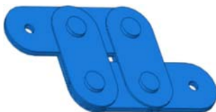
Fig. 47. Rotary friction damper
