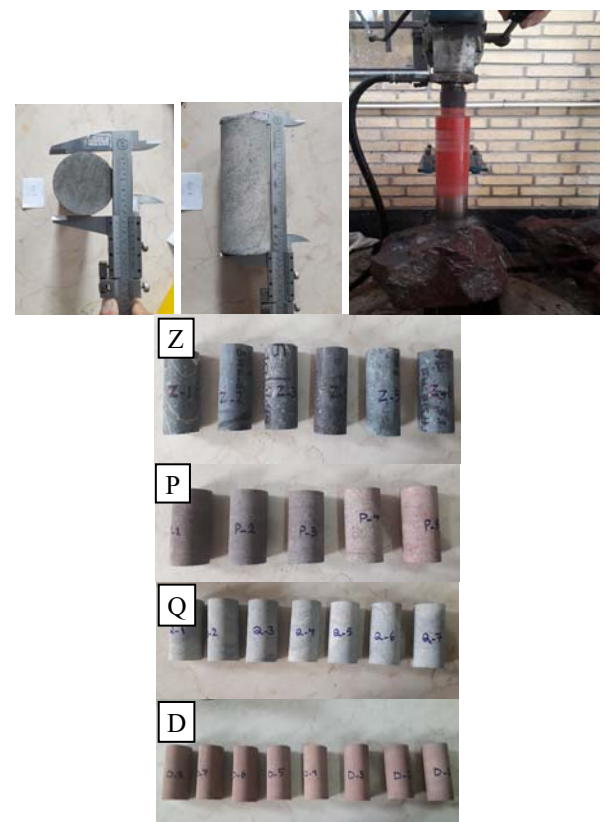
Fig. 7. Coring and measuring the dimensions of the prepared samples (up), Cylindrical specimens prepared: zanjan trachyandesite (Z), parand andesite (P), Qazvin latite (Q), Damavand sandstone (D), (down).
