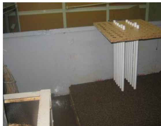
Fig. 5. SFM structure after installation in the reservoir
