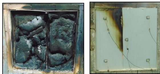
Fig. 14. Exposed surface (left) and unexposed surface (right) of PIR SWP-A after test
