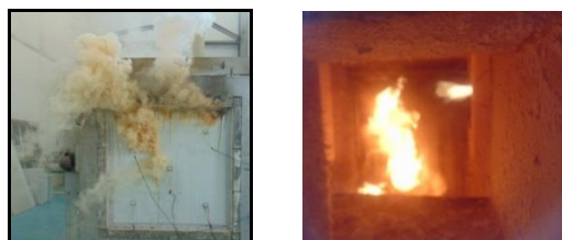
Fig. 7. PUR SWP-M1 during fire resistance test
