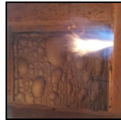
Fig. 11. Unexposed surface PIR SWP-M3 after test
