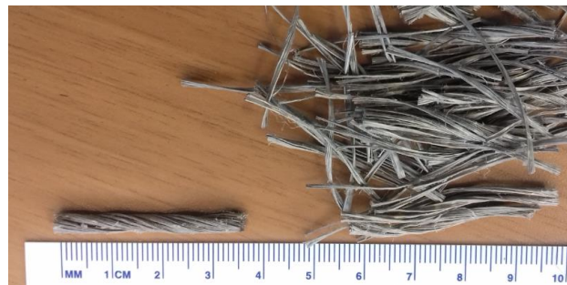
Fig. 2. The Twisted bundle polypropylene fibers used in this research
