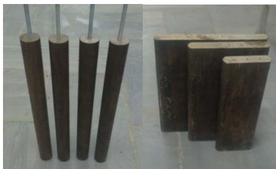
Fig. 3. Different shapes of piers
