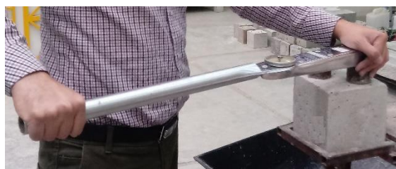
Fig. 3. "Twist-off" in-situ Test.
