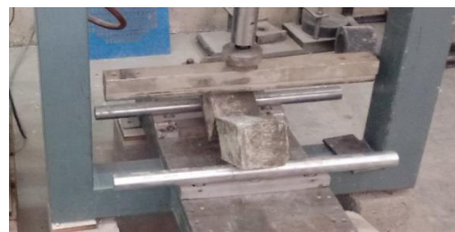
Fig. 4. "Flexural Strength" Test.
