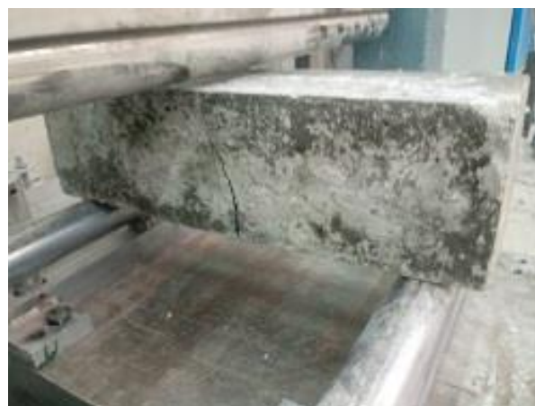
Fig. 17.a. Fracture of concrete containing fibers
