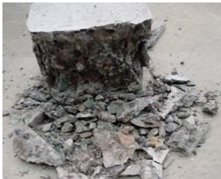
Fig. 15.b. Fracture of concrete Without fibers
