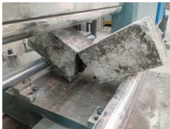
Fig. 17.a. Fracture of concrete Without fibers
