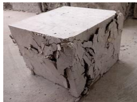
Fig. 15.a. Fracture of concrete containing fibers
