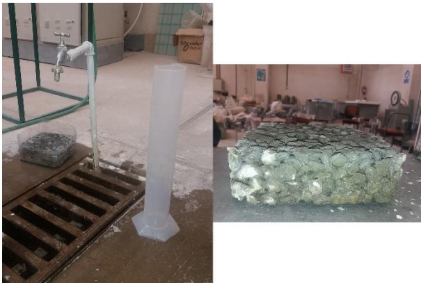
Fig. 3. Permeability test on pervious concrete
