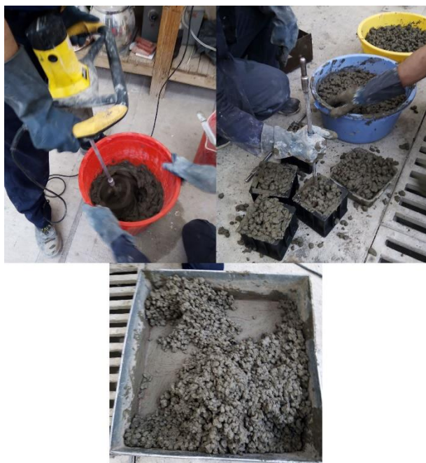
Fig. 2. Production of pervious concrete
