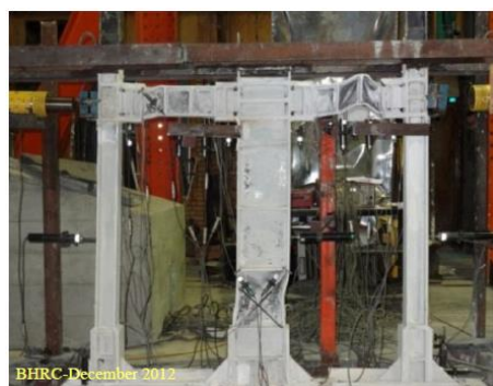
Fig. 8. The experimental sample of prismatic TRF for verification purpose[23]
