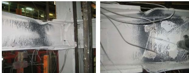
Fig. 7. EXD-1 specimen at the end of test and drift story  $6\%$
