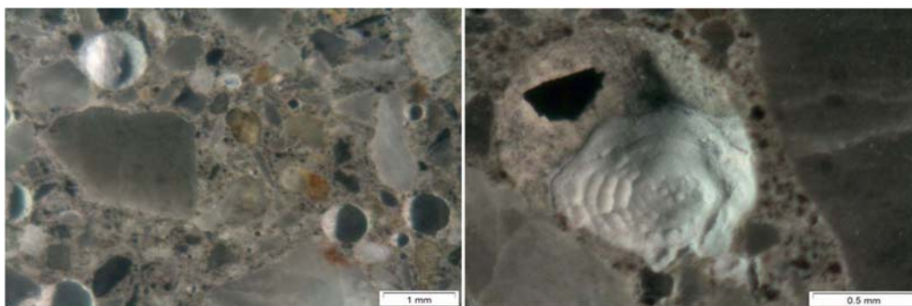
Fig. 6. Alkali-silica gel Formation in the Concrete Sample without Pozzolan
