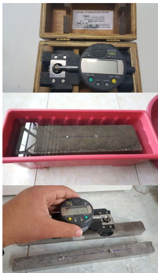
Fig. 1. Measuring length change of concrete and cement paste
