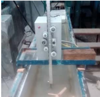
Fig. 7. The Bed Profiler and its placement position in channel
