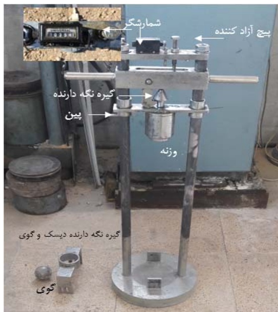
Fig. 3. Drop-Weight Impact test machine
