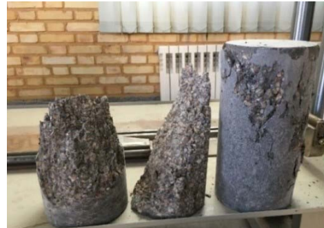
Fig. 4. Fracture pattern of concrete under compressive test a) Plain concrete b) steel fiber-reinforced concrete
