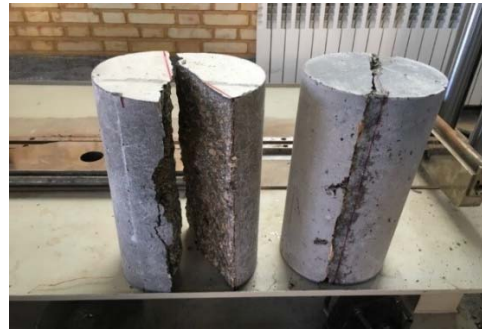
Fig. 7. Fracture pattern of concrete under tensile test a) plain concrete b) steel fiber-reinforced concrete
