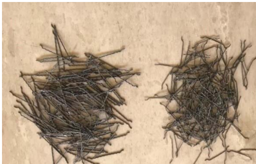
Fig. 1. Shape of the wavy hooked-end steel fibers used in the study
