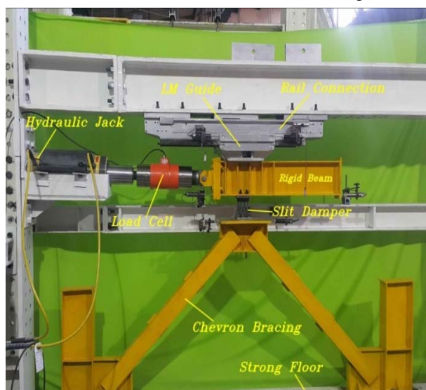
Fig. 3. Test layout system and the installations
