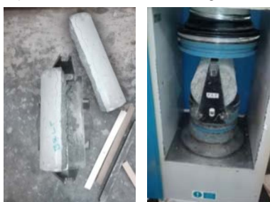
Fig. 16. Tensile strength test layout
