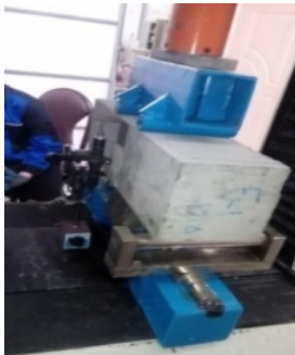
Fig. 18. bending strength test sample
