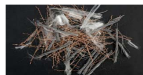
Fig. 3. Shape of crimped- end hooked steel and modify polypropylene fibers
