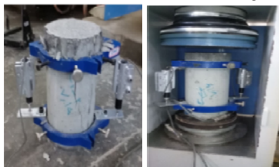
Fig. 14. Compressive strength test sample
