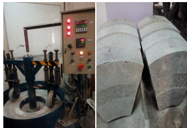
Fig. 2. Abrasion resistance test machine and specimens
