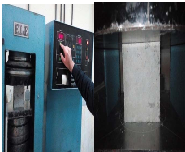
Fig. 1. Compressive strength test machine and specimen
