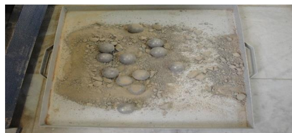
Fig. 11. Material after Los Angeles test
