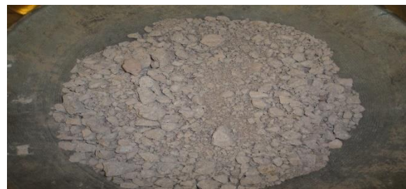
Fig. 10. Material after Oedometer test
