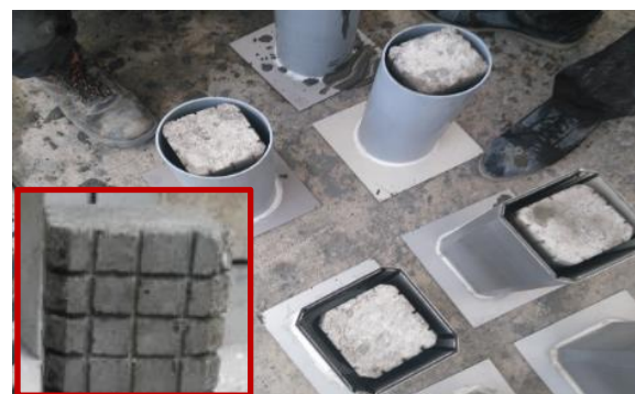
Fig. 1. Implementation of grooves and cover layer
