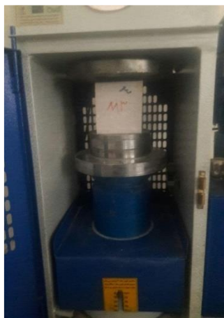
Fig. 4. Testing the compressive strength of the samples
