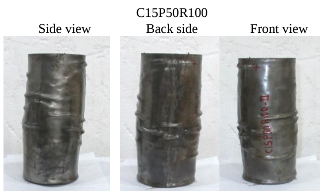
Fig. 8. Failure mode of column, 50 bar external pressure, 15 MPa concrete, D/t=100
