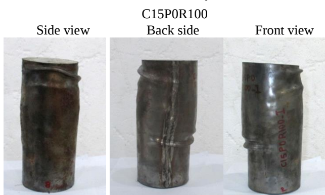
Fig. 7. Failure mode of column without external pressure, 15 MPa concrete, D/t=100
