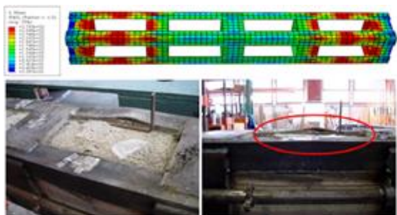
Fig. 22. Failure modes observed in the FE and experimental model [13]
