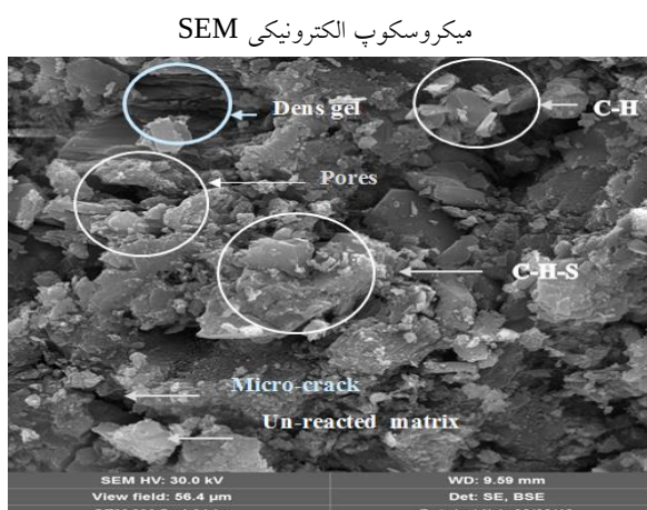
Fig. 11. SEM Images of control sample
