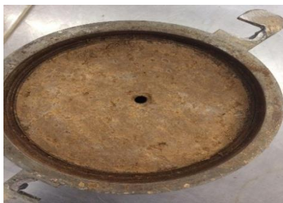
Fig. 5. Schematic of Hole in the standard compaction mold
