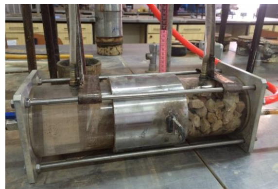
Fig. 4. Photograph of hole erosion device used in this research
