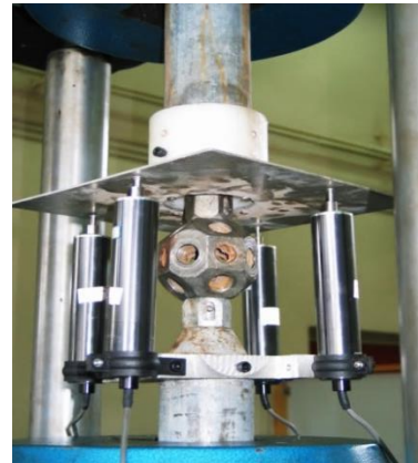
Fig. 5. Experimental model of Mero joint under tensile load [16].
