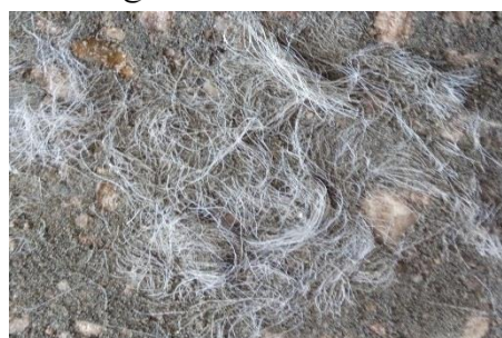
Fig. 6. Flattening of fiber at concrete surface
