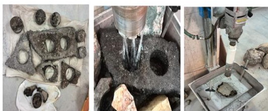
Fig. 2. Coring the asphalt concrete in the laboratory.
