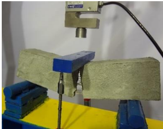
Fig. 10. Crack bending stitching by fibers
