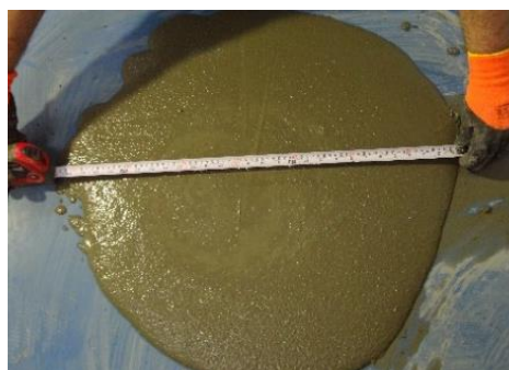
Fig. 3. Flow slump test
