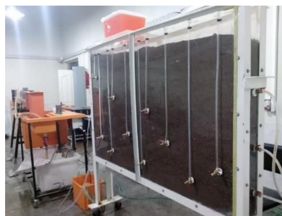
Fig. 1. Experimental model for contaminant transport in porous media
