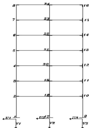
Fig. 12. Applying displacements to structural support in SAP 2000 software
