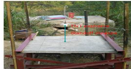
Fig. 5. Test setup slab under blast load
