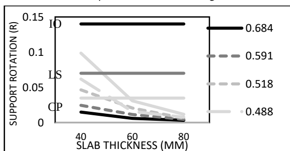
Fig. 18. Rotation of support's plastic higs and performance level of slabs without WM, 50MPa
