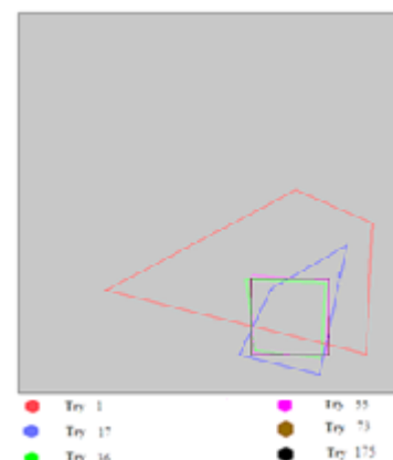
Fig. 9. Determination of geometry of regular hole in 2D plate at static analysis
