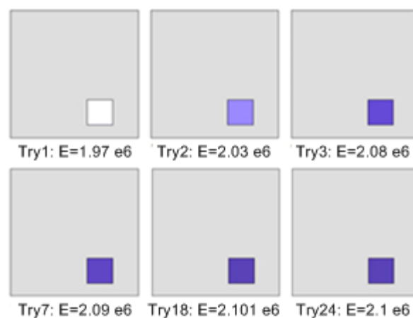
Fig. 13. Determination of elasticity modulus in dynamic analysis in 2D plate with regular hole
