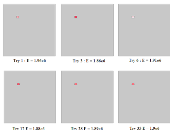
Fig. 15. Determination of elasticity modulus in dynamic analysis in 2D plate with irregular hole
