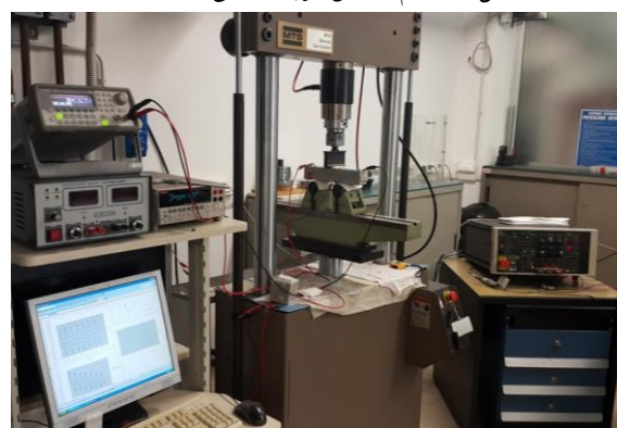
Fig. 1. Three points bending fatigue test setup
