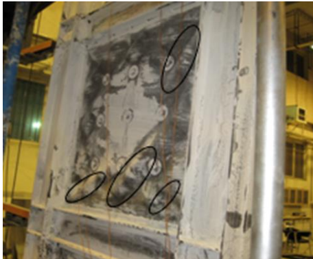
Fig. 19. Out of plane deformation of composite shear wall model without opening [6]
